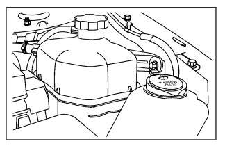
The surge tank is located on the driver's side of the engine compartment. See *Engine Compartment Overview on page 314* for more information on location.
